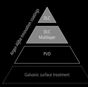
Argor-Aljba's ta-C DLC coatings, due to their tetrahedral structure, acquire the properties of a diamond. The share of the sp3-configured carbon lies around 75-85%, which is the reason for the high content of diamond structure. Furthermore, due to its procedure, Argor-Aljba's ta-C coatings are completely free of hydrogen.
